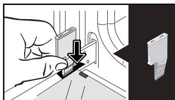
Remove the first clipped glass panel: Using the other wedge (or a screwdriver), press into the slots A to unclip the glass. Remove
