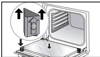
After cleaning, reposition the four rubber stops with the arrows upwards and reposition all of the glass panels.
