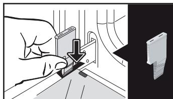
Remove the first clipped glass panel: Using the other wedge (or a screwdriver), press into the slots **A** to unclip the glass.
