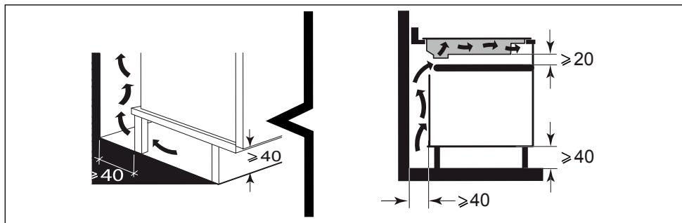
or above a built-in oven, comply with the dimensions provided on the illustrations to ensure a sufficient outlet air flow.
